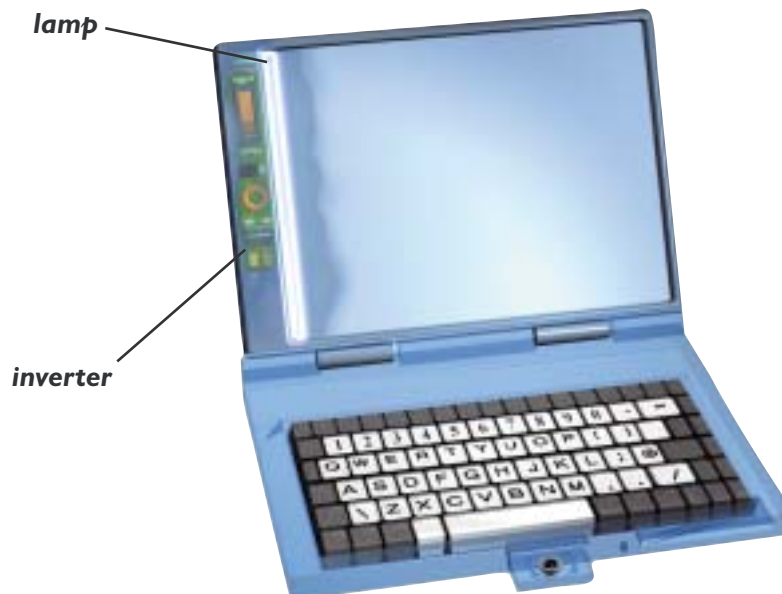
Fig.2 Example of Notebook computer with LCD backlighting
