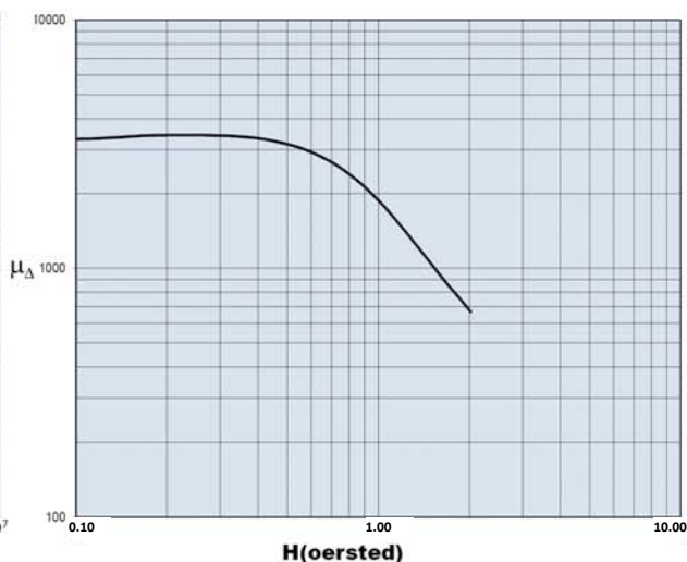
Incremental Permeability vs. H
