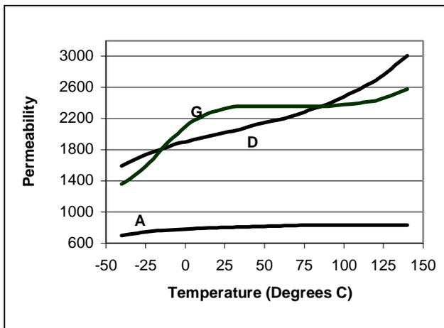
**Figure 9.** The low level materials are engineered for filter applications. **G** is quite flat in the 20°C to 70°C range. **A** is fairly flat in a wider temperature range. **D** is linear, with a temperature factor ( $T_F$ ) to match that of some capacitors. See the ferrite catalog (FC-601) for  $T_F$  data and design notes.
