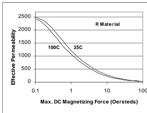
**Figure 11.** Maximum DC Bias for gapped ferrite cores.
