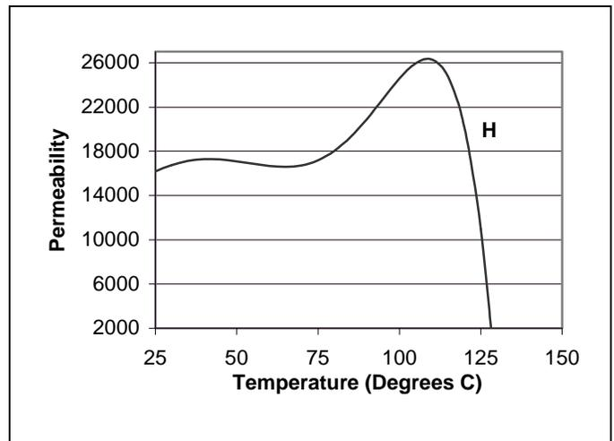
**Figure 4.** H material Curie temperature is 120°C
