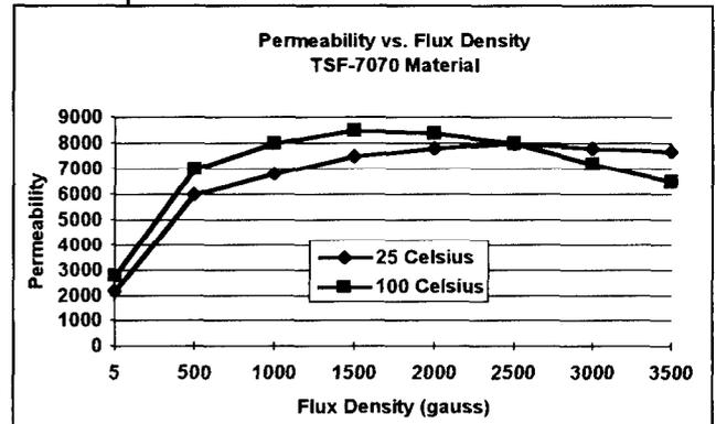
Permeability varies with flux density and temperature, hence the measured inductance also changes with changes in flux density and temperature. Therefore, the flux density and temperature must be controlled. To calculate the test voltage for a given flux density, the following formula is used:
